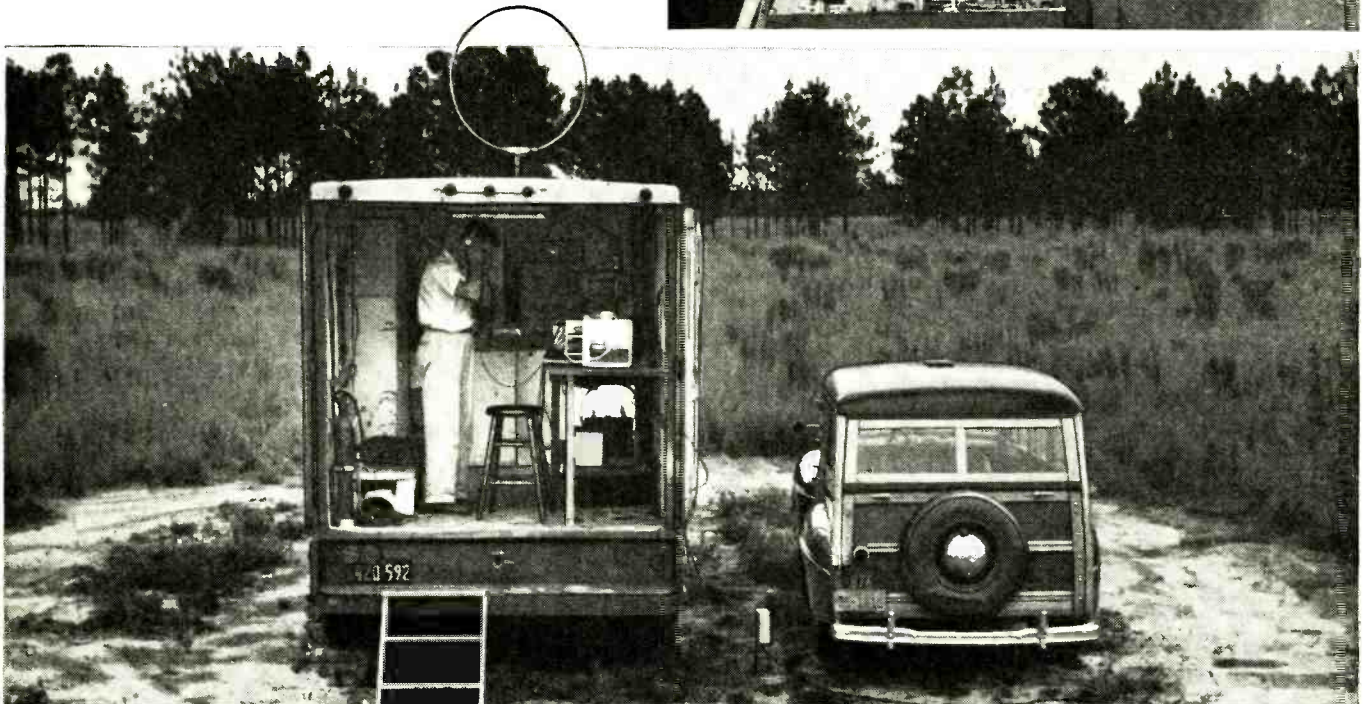
Thunder hunting equipment on location near Madison, Florida. Loop antenna on truck picks up static. The engineer in top picture is watching the indication of a circuit which registers how often the static exceeds a given level.
